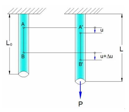
Figure 3.1 Axially loaded bar
