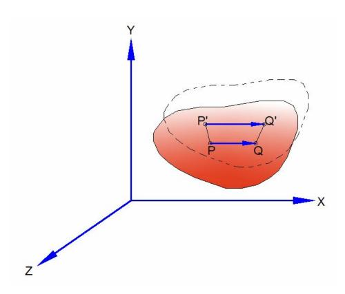
Figure 3.3 Line element in undeformed and deformed body
